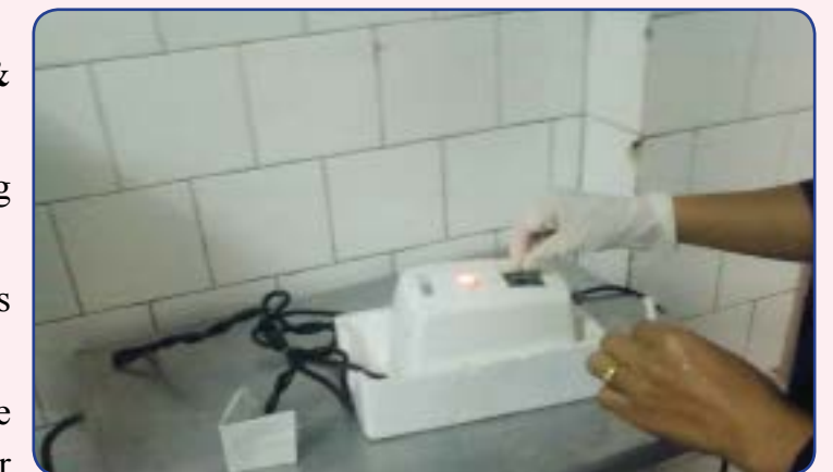
An electric needle destroyer in which needles &amp; syringes are destroyed
