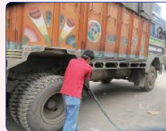
Emission test of Diesel vehicle in progress
